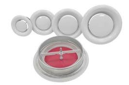
Polyaire's Fire Rated Air Valves are a unique and cost effective fire rated solution where recessed ceiling air valves are to be installed in fire rated floor/ceiling constructions. In a fire situation, the integral intumescent material rapidly expands to seal off the air valve to help maintain the fire resistance rating of the ceiling. This limits the risk of fire and heat spread throughout the building.
